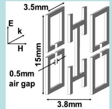
FIG 2 Structural details of the negative- $n$  material
