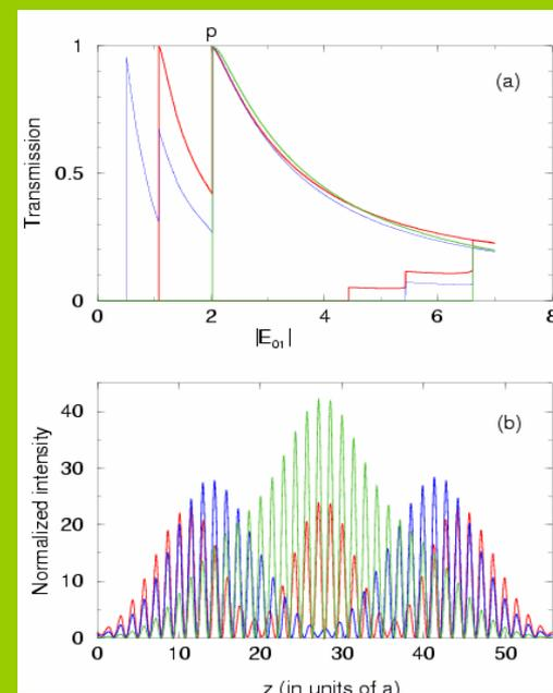
Fig. 1 shows a typical MFGS in a 1D NCP possessing three frequencies inside the gap. (a) Transmission as a function of incident amplitude from three beams at different frequencies (in red, blue, and green) The amplitudes of three beams are kept at fixed ratios. (b) Intensity distributions at Point P for the respective frequencies.
