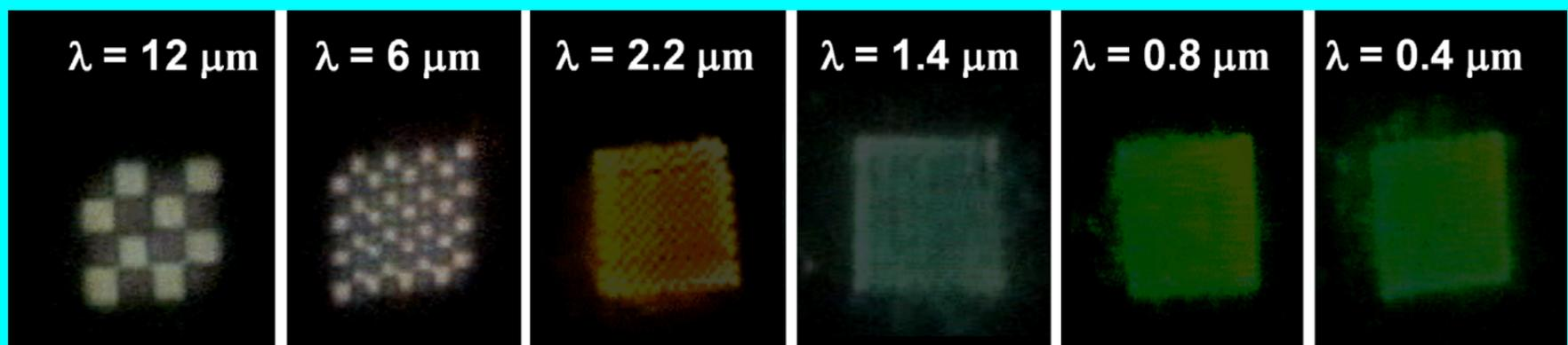
Fig. 2 Optical images of LC cells constructed with one side made of the substrates illustrated in Fig. 1 and the other side ITO/glass coated with polyimide rubbed along  $y$ . The images were taken with the LC cells placed between crossed polarizers with the entrance polarizer oriented along  $y$ . An inhomogeneous-to-uniform LC alignment transition near  $\lambda = 0.8 \mu\text{m}$  is readily apparent from these images. Please refer to Ref. 2 for more details.
