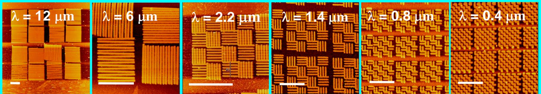
Fig. 1 Atomic force microscopic (AFM) topographical images of the nano surface patterns used in this study for the control of LC alignment. The patterns were fabricated by the AFM local oxidation method [1]. The scale bars represent 3  $\mu\text{m}$ .
